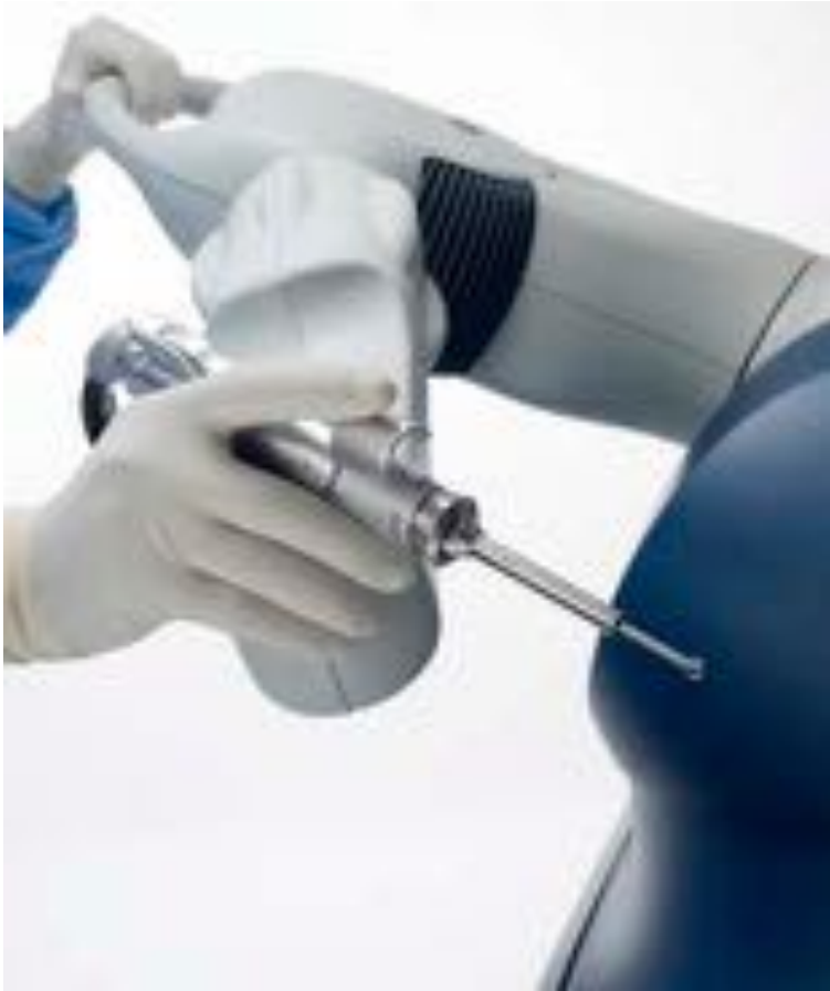
Mako's RIO Robotic Arm Interactive Orthopedic System
