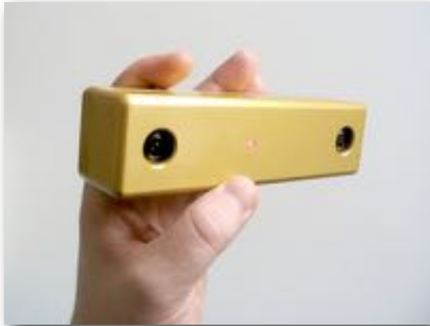
Bumblebee Firewire Stereo Vision Camera
