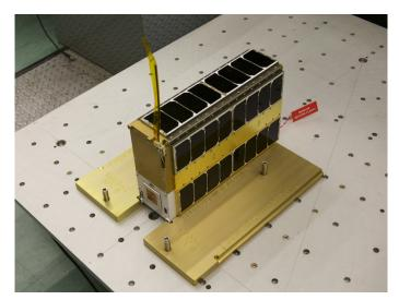
Figure 4: EcAMSat FLT-1 undergoing mass properties evaluation
