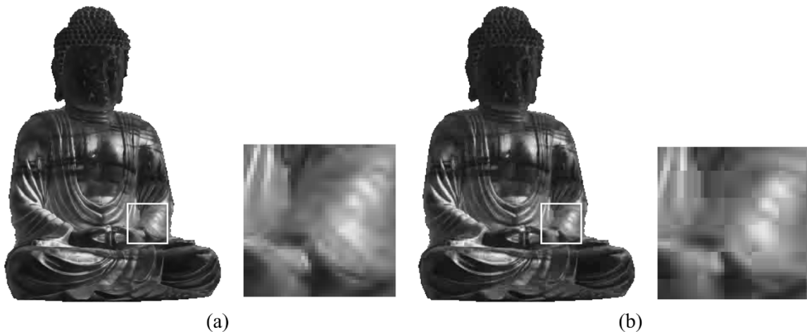
Fig. 14. Luminance component of Buddha : The reconstructed view from different coders, corresponding to the labeled points on the rate-PSNR curves in Fig. 10, are shown with the white box labeling the area magnified beside. (a) Proposed at 0.297 bpop. (b) SA-DCT at 0.296 bpop.
