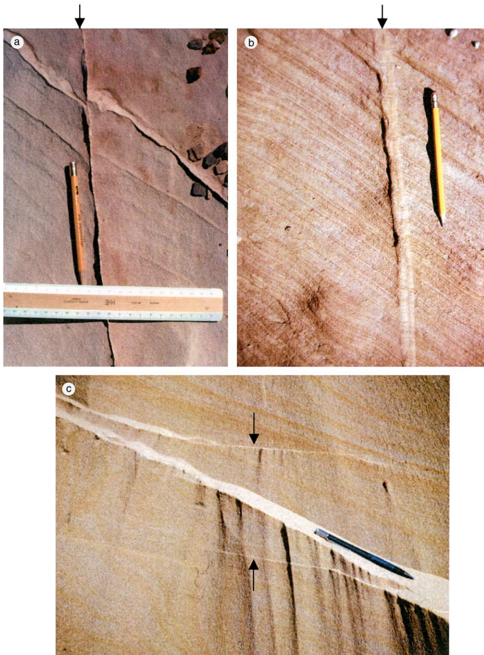
Fig. 2. (a) A shear band (marked by arrow) in the Entrada Sandstone, San Rafael Desert, Utah. The band is about 1–2 mm in thickness and displaces nearly horizontal beds by a few mm (left-hand side down). Ruler is about 20 cm long. (b) A compaction band in the Aztec Sandstone at Valley of Fire, Nevada. The band is about one cm thick, has no observable shear offset across it, and shows significant porosity decrease. Standard size pencil is for scale. (c) Dilation bands (nearly horizontal traces marked by arrows) in unconsolidated terrace sand near McKinleyville, Northern California. Pencil on the surface of the shear band is for scale. Porosity distribution across a thin section covering a horizontal band indicates about 7% porosity increase within the band.
