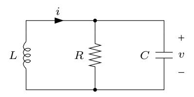
$$\sigma = \frac{-1}{2RC}, \quad \omega = \sqrt{\frac{1}{LC} - \frac{1}{4R^2C^2}}$$
