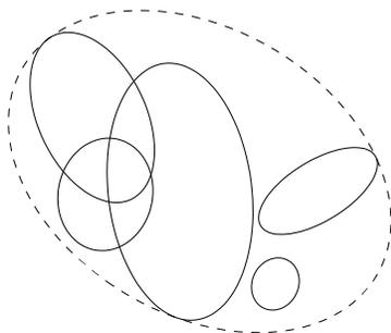
**Figure 2** Minimum volume ellipsoid containing five given ellipsoids. Finding such an ellipsoid can be cast as a maxdet-problem, hence efficiently solved.
