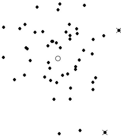
**Figure 3** A  $D$ -optimal experiment design involving 50 test vectors in  $\mathbf{R}^2$ . The circle is the origin; the dots are the test vectors that are not used in the experiment (*i.e.*, have a weight  $\lambda_i = 0$ ); the crosses are the test vectors that are used (*i.e.*, have a weight  $\lambda_i > 0$ ). The  $D$ -optimal design allocates all measurements to only two test vectors.
