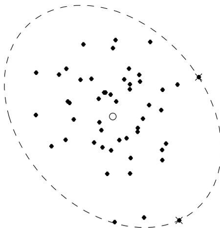
**Figure 4** In the dual of the  $D$ -optimal experiment design problem we compute the minimum-volume ellipsoid, centered at the origin, that contains the test vectors. The test vectors with a nonzero weight lie on the boundary of the optimal ellipsoid. Same data and notation as in Figure 3.
