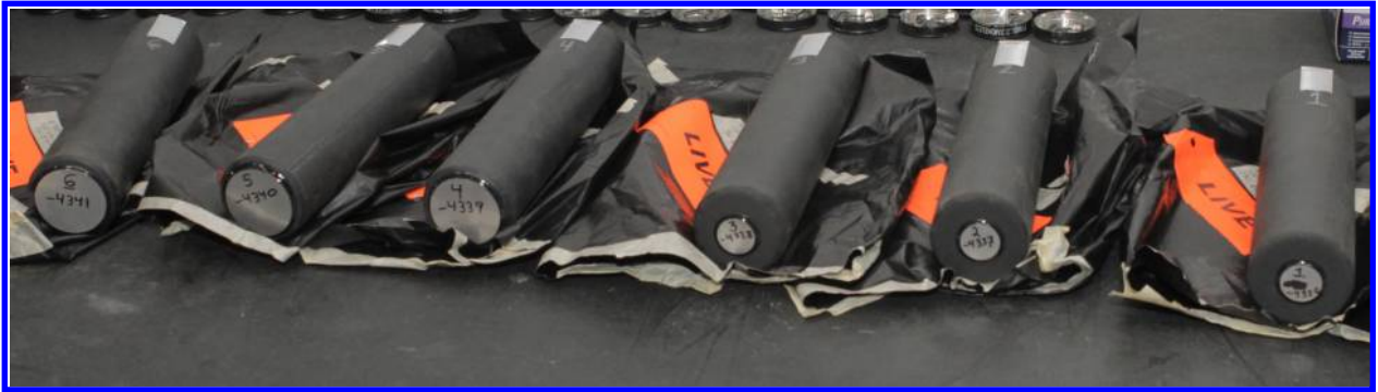
Fig. 13 End-burning “insulated log” analog samples.
