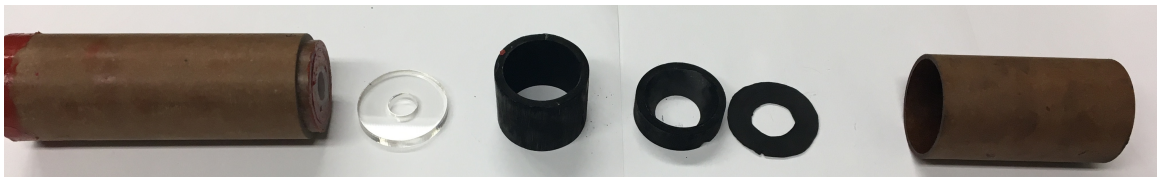
Figure 3.10: Most of the components used inside the combustion chamber are consumable. The only parts used in multiple tests are the graphite post combustion chamber and the graphite ramp, which transitions the flow from the combustion chamber diameter to the entrance diameter of the nozzle.
