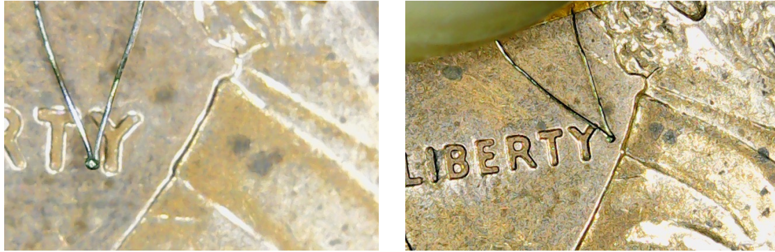
Figure 4.7: Two thermocouple junctions are shown on top of a penny. The penny is used as a scale reference to illustrate how small the fabricated sensors really are. These sensors are made by welding two 50\ \mu\text{m} wires together.
