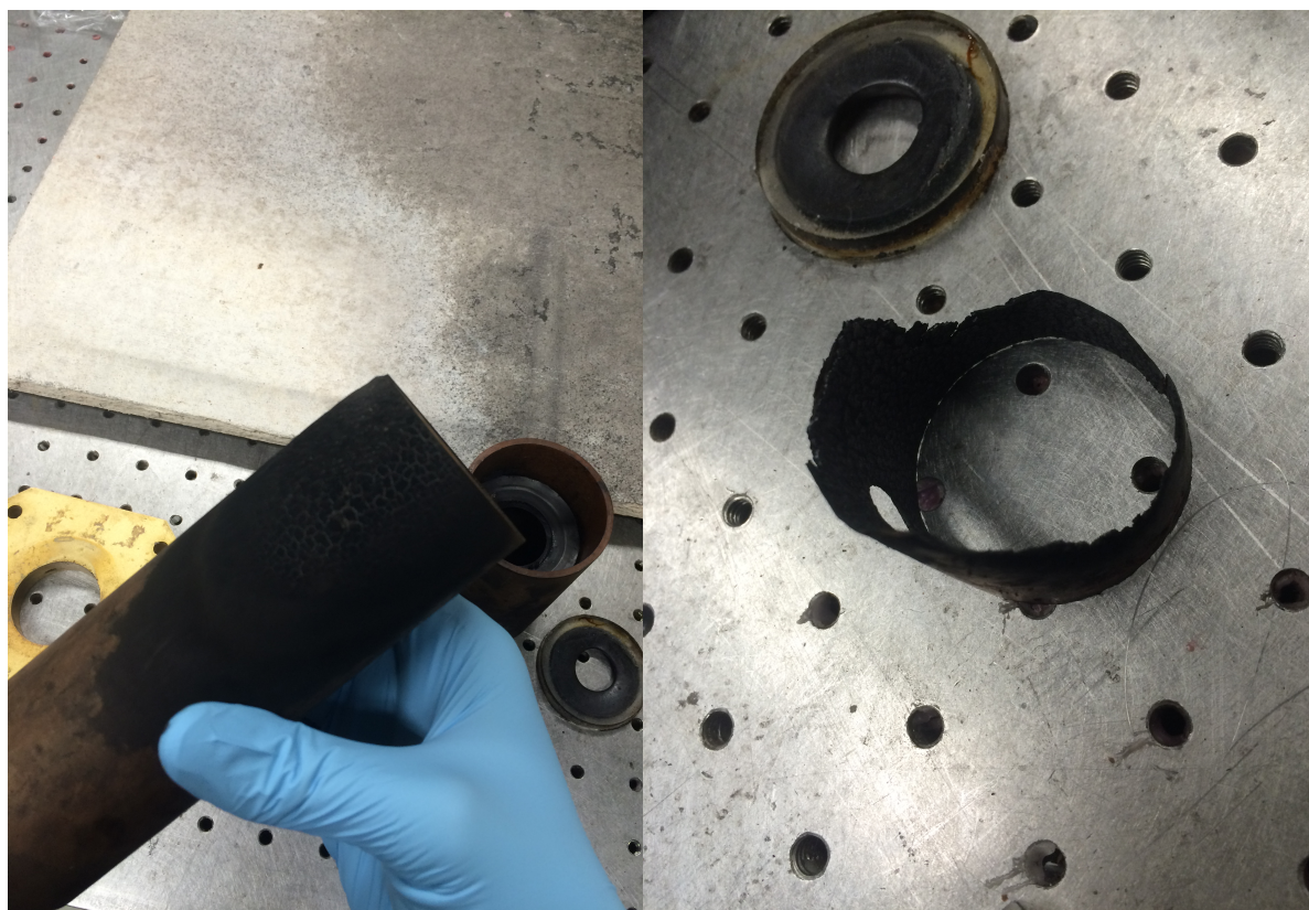
Figure 5.16: The outside of the fuel grain insulator (left) was accidentally burned as well as the fore end insulator (right). The pre-burning of the oxidizer with the fore-end insulator likely led to increased efficiency of the burn.
