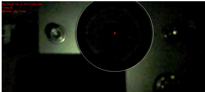
Figure 7.2: The upscaled calibration image shows that the fore end support block of the motor has a viewport diameter of 324 pixels, which corresponds to 5.07 cm. To measure the fuel grain diameter, a correction factor of 1.039 is applied to account for perspective losses because the fuel grain is further away from the camera lens.
