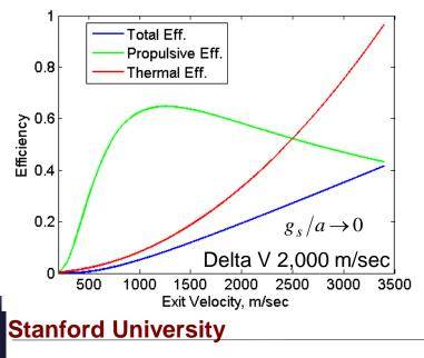
Even though the propulsive efficiency is maximized at a certain exhaust velocity, the product of the propulsive and thermal efficiencies increases monotonically with increasing exit velocity (i.e. specific impulse).
