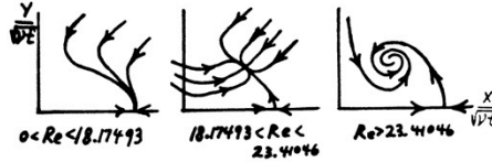
Figure 9. Entrainment diagrams of H(\xi, \theta) (equation 55) for various Reynolds number ranges.
