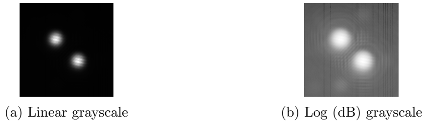
Figure 6-7: Tight-packed symbol CH(6,3) on linear and log grayscale The image is taken as the average of ten shots of the static profile CH(6,3) profile, from which an averaged background from fifty images is subtracted. For the logscale image, averaged pixel values under one are rounded up to one. The highest pixel value is used in determining the grayscale range.
