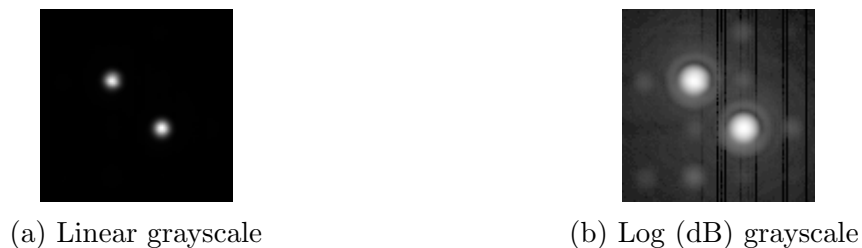
Figure 6-2: CCD image of symbol CH(6,3) on linear and log grayscale. The image is taken as the average of ten shots of the static profile CH(6,3) profile, from which an averaged background from fifty images is subtracted. For Figure 6-2b, averaged pixel values under one are rounded up to one to ensure the log scale behaves well. The highest pixel value is used in determining the grayscale range.
