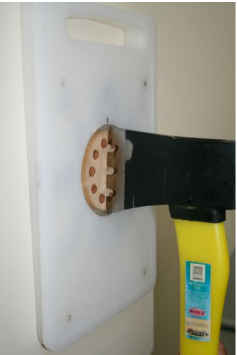
Fig. S2. To avoid carrying surface material into the interior of wood disk, we split the disk first with a triple-notched, straight-ground edge axe (A-Xenic Extractor; AXE) into two parts and then split each half radially three more times with a single-notched chisel. We then drilled eight sawdust samples from the exposed wood surface on the interior of disk underneath the notched portion of the splitting devices. The middle notch under the AXE sampler was not used for this experiment. (Note that here a non-inoculated, dry wood disk used for illustration purposes).
