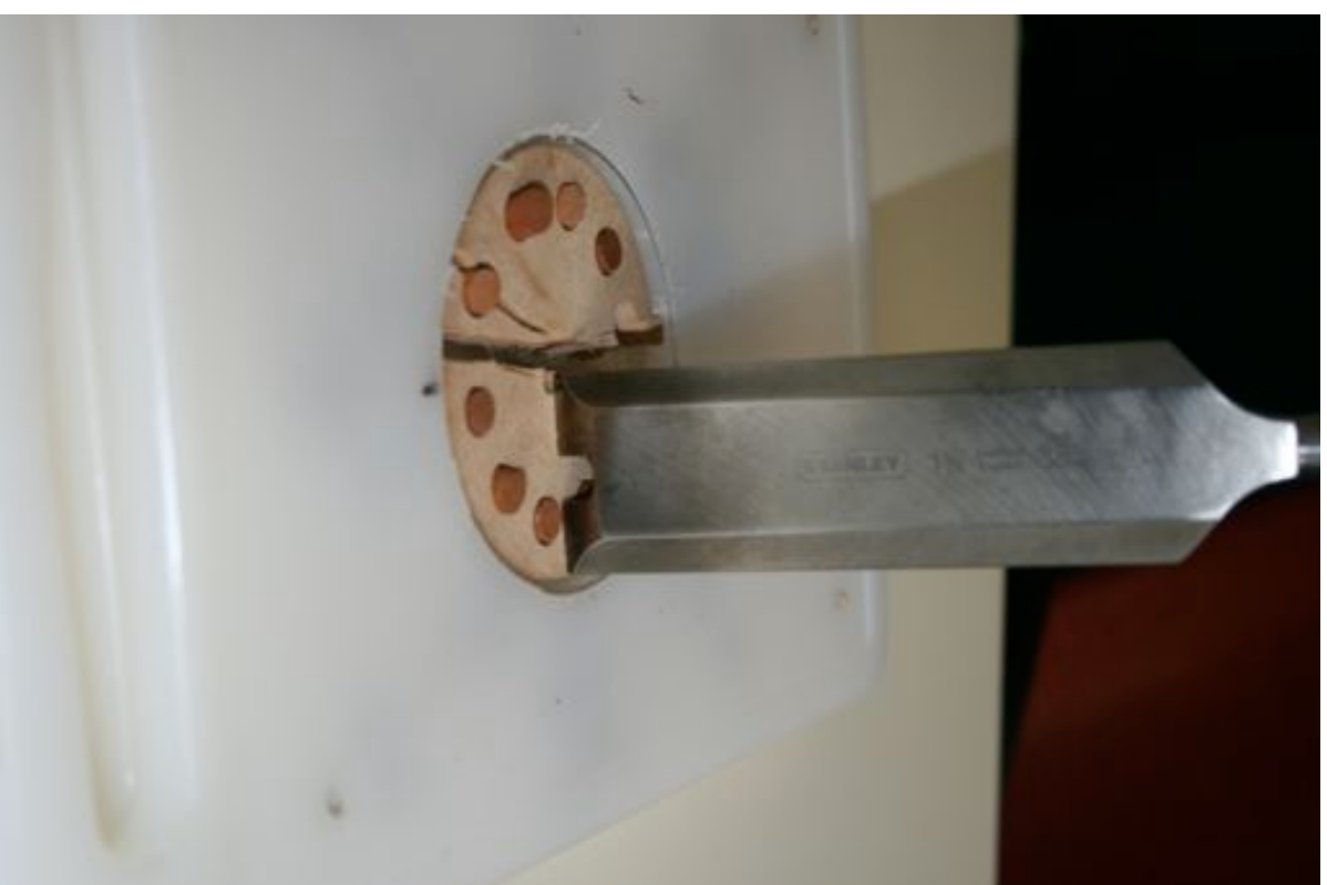
Fig. S2. To avoid carrying surface material into the interior of wood disk, we split the disk first with a triple-notched, straight-ground edge axe (A-Xenic Extractor; AXE) into two parts and then split each half radially three more times with a single-notched chisel. We then drilled eight sawdust samples from the exposed wood surface on the interior of disk underneath the notched portion of the splitting devices. The middle notch under the AXE sampler was not used for this experiment. (Note that here a non-inoculated, dry wood disk used for illustration purposes).
