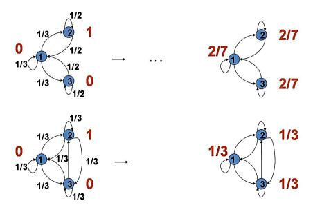
**Figure 5.2.** The DeGroot updating process for two different configurations: In the top setting agents 2 and 3 are not friends and the process is slower to converge to a consensus, in the bottom setting there is a complete network and consensus occurs in the first period.
