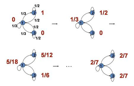
**Figure 5.2.** The DeGroot updating process over time for the system in Figure 5.2 when agent 2 starts with belief 1 and the other agents start with belief 0.
