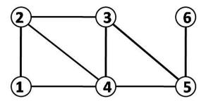
**Figure 3.3.1.** Clustering is 1 for nodes 1, is 2/3 for nodes 2 and 3, is 1/2 for node 4, 1/3 for node 5, and 0 for node 6
