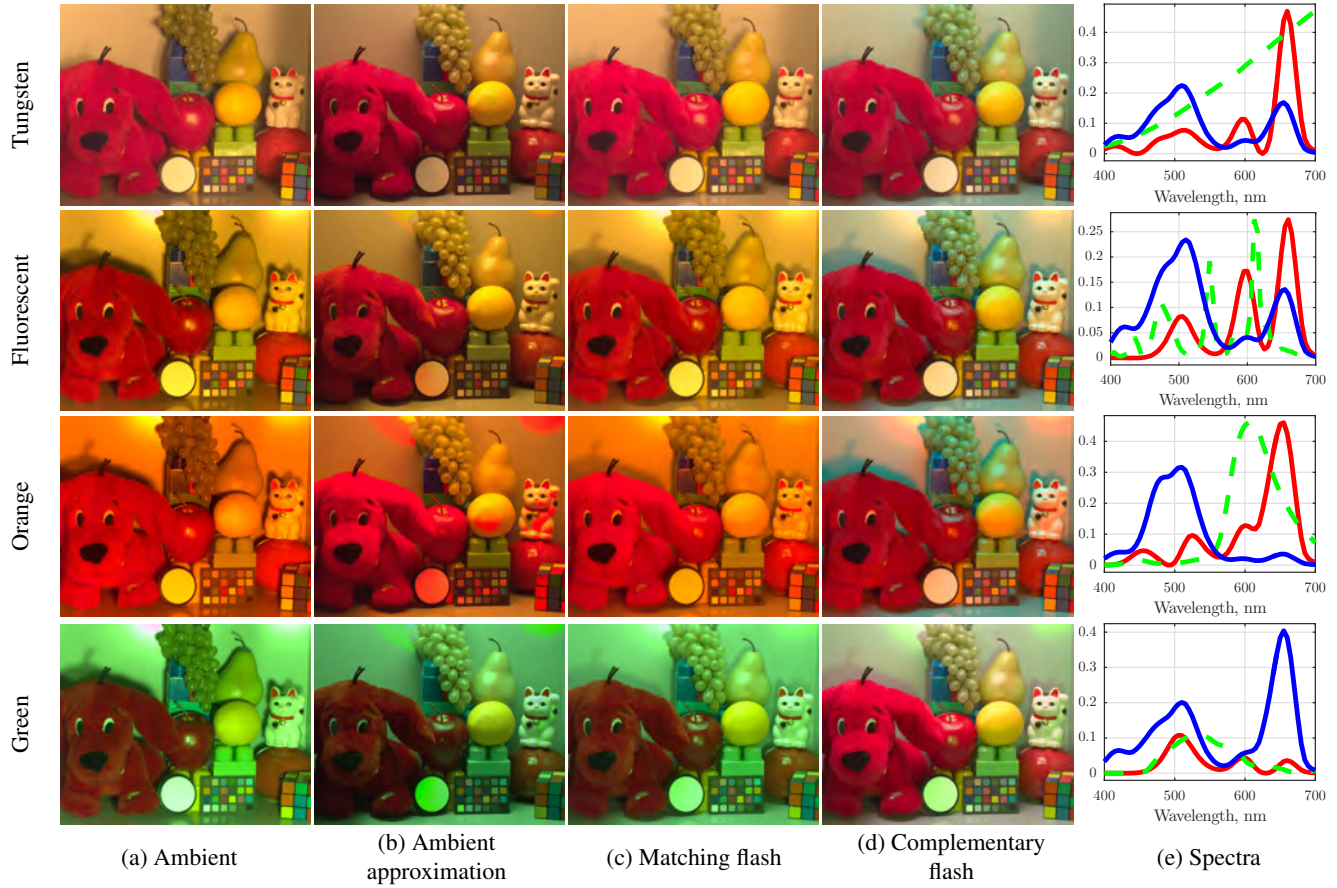
Figure 8. Computational spectral flash can adjust its spectral power distribution to deliver light that is similar ( matching mode) or that delivers the wavelengths that are missing ( complementary mode) from the ambient. Each row represents a different ambient illumination condition. Columns represent the ambient image (a), its linear approximation with narrowband light images (b) and images captured with the computational flash in the matching (c) and complementary (d) modes. Curves in (e) show the illuminant spectral power distributions of the ambient (green, dashed), estimated ambient (red) and the ambient complement (blue).
