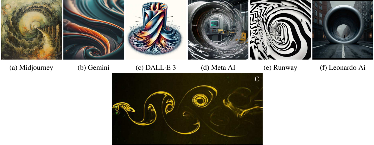
(g) Von Kármán vortex street behind an oscillating circular cylinder in a lab experimental setup; this image is taken from part (c) of Fig. 25 in Khan et al. [2023], published as open access under a Creative Commons license in the Journal of Fluid Mechanics, allowing readers to distribute the content freely.
