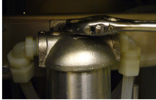
Fig. 4. The water filter is contained inside the canister, and can be extracted by loosening the nut on the top. To gain access to this part of the machine, a front panel must be removed.
