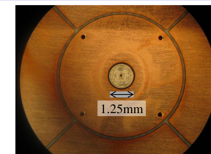
A single-mode fiber is introduced through the center via of the innermost electrode (actually a fiber ferrule).
