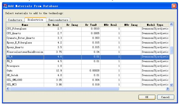
Now we should see the dielectric material only have one kind that is FR-4. Press OK to confirm and go back to the layer view. Then choose FR-4 in the drop-down box of material.
