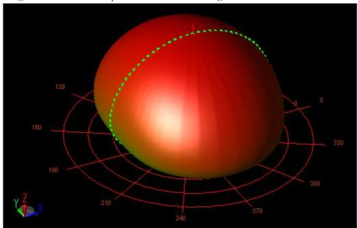
Now you can choose 'Plot Properties' tab at left bottom side, choose 'Far Field Cut' tab above, click 'Enable'. Adjust  $\theta$  and  $\phi$  values to choose your cut, then press 'Display Cut in Data Display' to see the profile of that cut.
