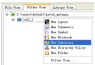
4. In substrate window, we can see a view of all the layers of our design. Click on them, you can see the material and thickness of each layer on the right panel. From top to
