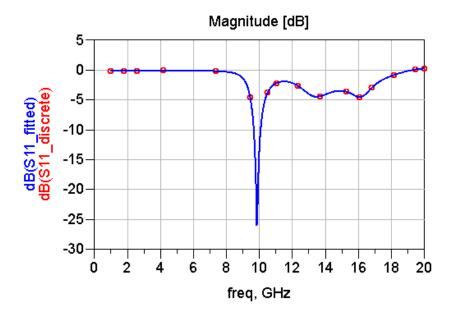
In the plot, we can see that frequency around 10GHz is all radiated out so its reflection is very small. At other frequencies, the S11 value are almost 0 namely S11=1, which means they are all reflected.
