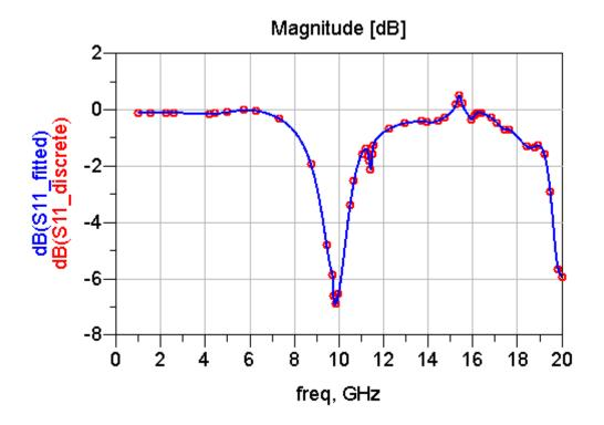
Here, we only have S11=-7dB compared to -25dB when feed line is recessed. This shows that a recessed feed line indeed decreased the input impedance so that antenna can be matched way better at 10GHz with much smaller reflection.
