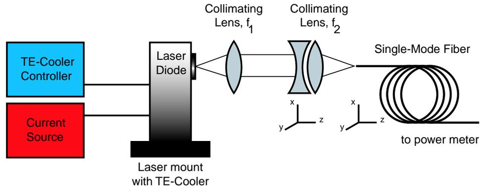
**Figure 2.** Setup for laser-to-fiber coupling experiment.
