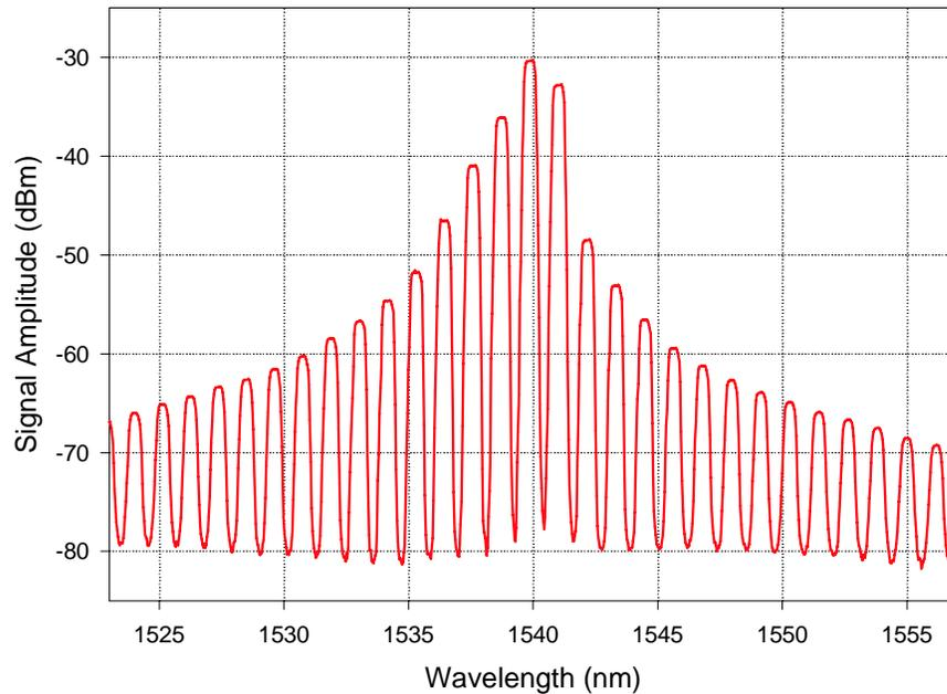
**Figure 3.** Spectrum of a Fabry-Perot laser diode as measured by an optical spectrum analyzer.
