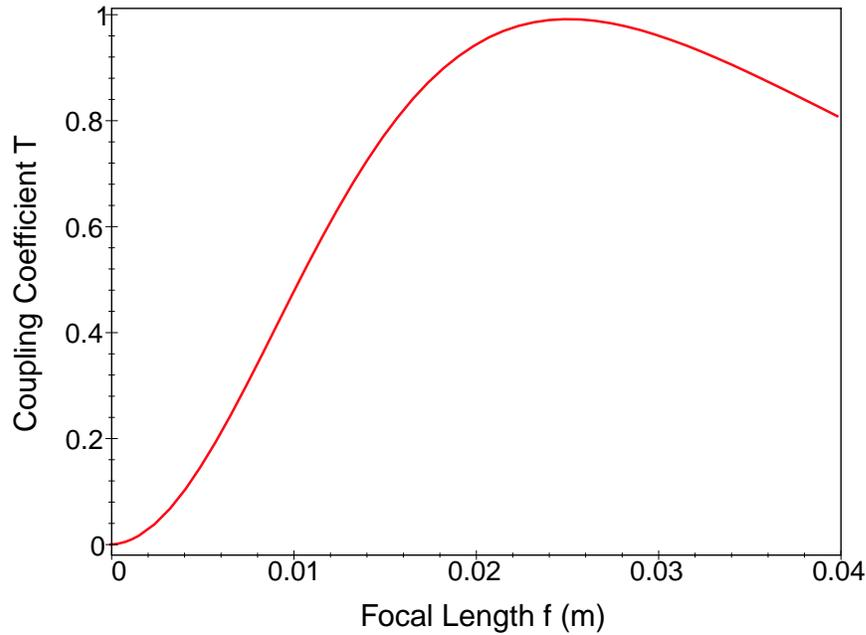
**Figure 1.** Coupling efficiency  $T$  as a function of focal length  $f$  for the case of modematching limited coupling.
