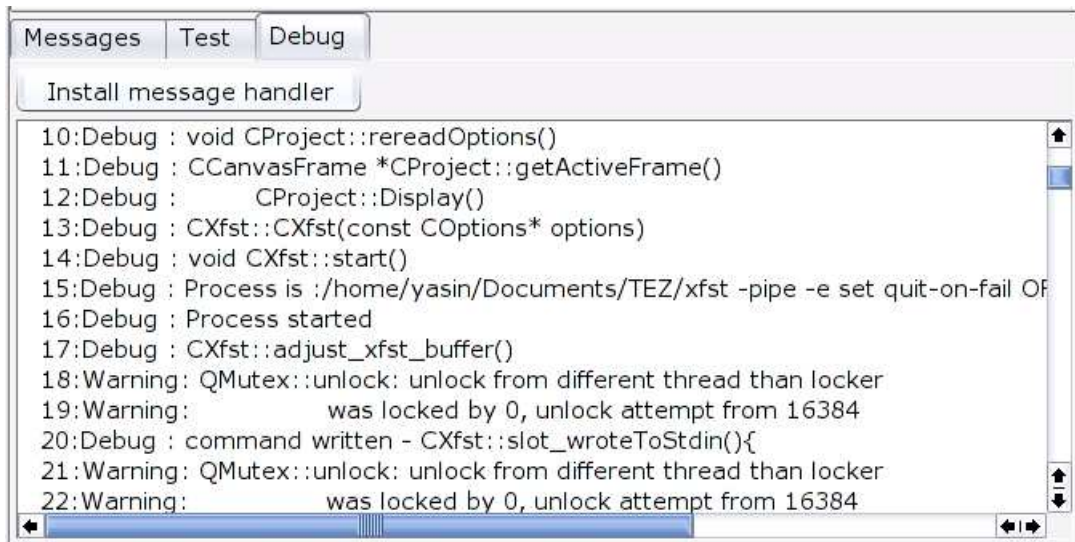
Figure 8: The debugging window is useful only when the debug option is set during compilation.
