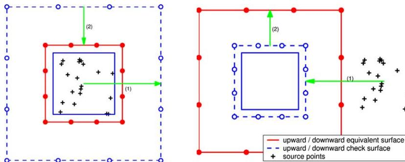
Fig. 4. The cross sections of the equivalent/check surfaces in 3D. Left: the upward equivalent density. Right: the downward equivalent density. In both plots, the innermost square is the source box. The equivalent and check surfaces are both discretized using the boundary nodes of a regular Cartesian grid. The nodes for the equivalent surfaces are marked with “●” and those for the check surfaces with “○”.
