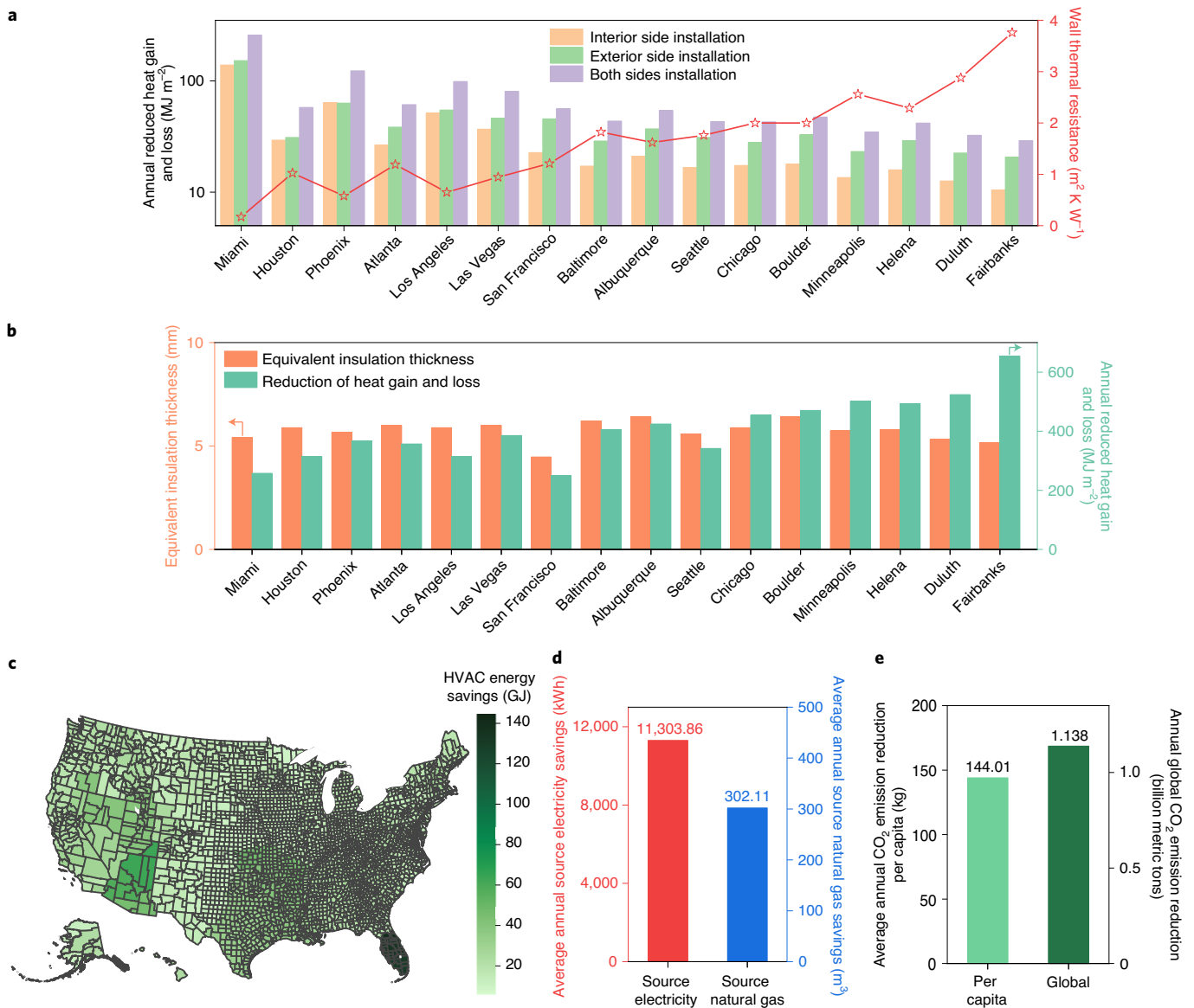
Fig. 5 | Modelled annual reduction of heat transmission and evaluation of building energy savings. a, Calculated annual reduction of heat gain and loss per installation wall area for installation on wall interior surface, exterior surface and both sides for 16 representative cities in various climate zones. b, Calculated equivalent insulation thickness for double-sided installation of coloured low-emissivity materials on non-insulated walls and its annual reduction of heat gain and loss per installation wall area. c, HVAC energy-savings map across the United States with coloured low-emissivity film installation on walls for a typical midrise apartment building. d, Predicted average annual source electricity and source natural gas savings for the modelled building. e, Predicted average annual CO 2 emission reduction per capita and globally.
