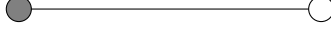
FIGURE 3. Example propagation graph used for illustration. Gray vertex denotes a sink. When a signal enters this vertex it is absorbed (a signal may exit the vertex, however). The edge is given the transfer function z^{-1} .
