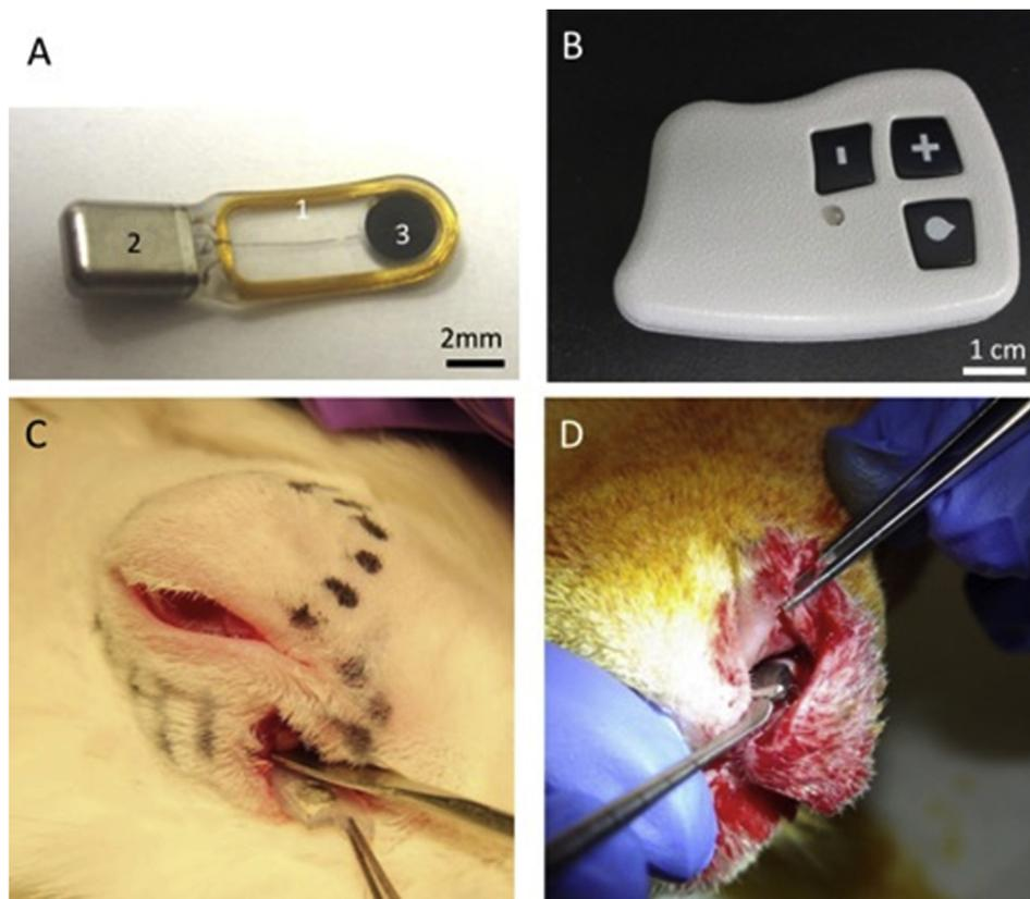
**Fig. 1.** A. Implant composed of the RF receiving coil (1), case with electronics serving as a return electrode (2), and an active electrode (3). B. RF power transmitter with adjustable pulse duration. C. Implantation near the lacrimal gland. D. Implantation into the nasal septum.
