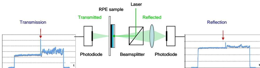
Fig. 1. Experimental setup for vaporization delay measurement. Delay was measured between the pulse onset and the first peak maximum for 6 incident powers between 160 and 640 mW.
