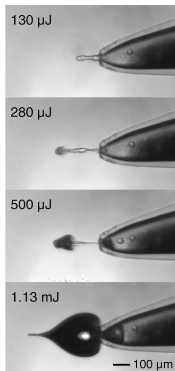
FIG. 3. Saline ejection into oil from a  $30\ \mu\text{m}$  nozzle driven by increasing discharge energies. Each frame is taken  $15.5\ \mu\text{s}$  after the electrical discharge. Note the appearance of hydrodynamic cavitation bubbles at high energies.
