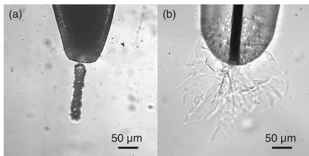
FIG. 4. Comparison of incisions in a polyacrylamide gel after a series of discharges from (a) the pulsed liquid microjet at 1.13 mJ/pulse and (b) the direct application of the plasma-induced vapor bubble at 0.14 mJ/pulse.
