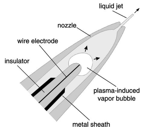
FIG. 1. Schematic diagram of the pulsed liquid microjet driven by expansion of a vapor bubble created by a submicrosecond high-voltage discharge.
