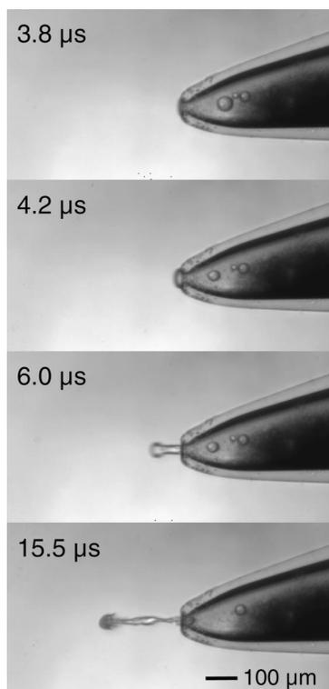
FIG. 2. Time sequence of saline ejection into oil from a  $30\ \mu\text{m}$  nozzle driven by a  $280\ \mu\text{J}$  discharge. Times noted on each frame correspond to delays after the electrical discharge.
