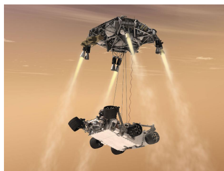
Fig. 1 Autonomous landing of the Curiosity rover on Mars using the Sky Crane maneuver. (Image credit: NASA/JPL-Caltech)
