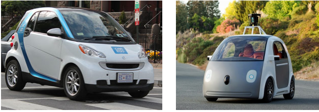
Fig. 1. Left figure: A Car2Go vehicle used in a traditional (i.e., non-robotic) MoD system. Right figure: Self-driving vehicle that Google will use in a 100-vehicle AMoD pilot project within the next two years. Image credit: Car2Go and Google.
