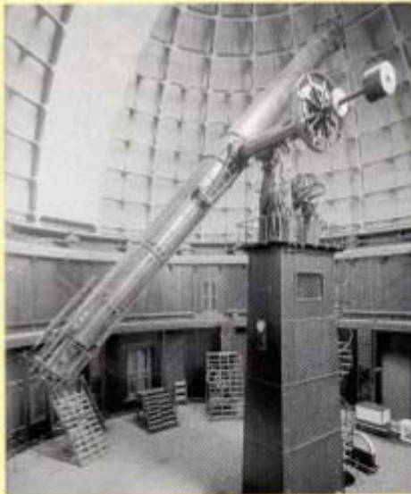
The Lick 36-inch refractor saw first light in 1888. One of the two lens blanks broke during transport, and it took some 18 attempts to make a replacement blank. This Clark telescope is still used today for infrequent research and public viewing.
