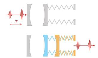
Top: A mirror is mounted on a spring and placed facing a second mirror. A photon in a superposition of two pulses (red) is fired at the mirrors. Bottom: Superposition state of the mirror on a spring both extending (blue) and compressing (orange) after being kicked by the photon at two different possible times.
