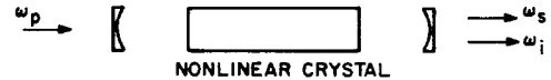
Fig. 1. Schematic of optical parametric oscillator. The mirrors are highly reflecting at either the signal or idler, or both.
