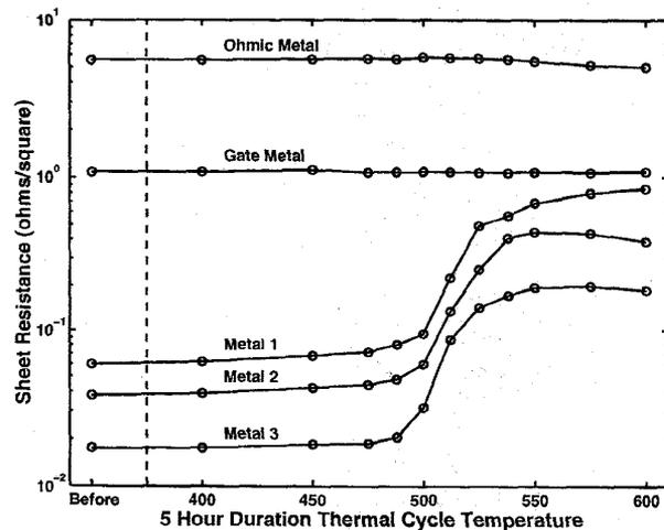
Figure 4: Metal layer sheet resistance after 5 hour thermal cycles. At elevated temperatures a metallurgical reaction,  $AlCu_x + WN_x \rightarrow Al-Cu-W-N$ , occurs within the interconnect metal layers which increases the sheet resistance.
