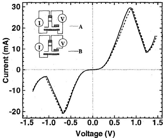
Figure 7: Current-voltage characteristics of a typical  $25 \mu\text{m}^2$   $\text{In}_{0.27}\text{Ga}_{0.73}\text{As}/\text{AlAs}$  relaxed-buffer RTD including and excluding the voltage drop contributed by the relaxed buffer.
