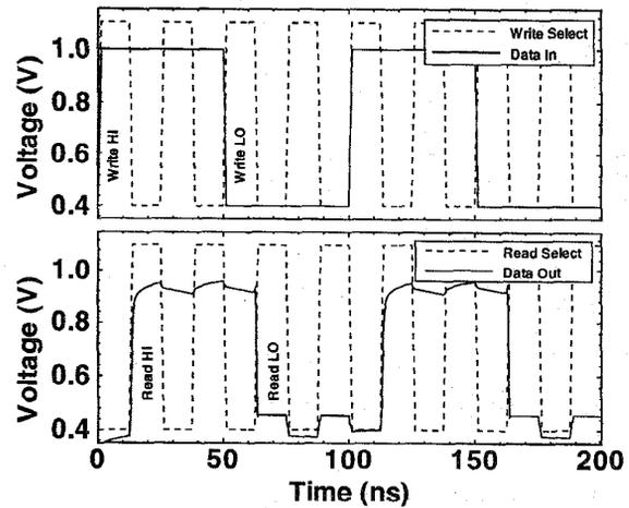
Figure 8: Simulated operation of 1-bit SRAM cell.
