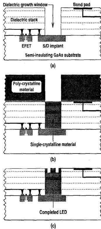
Figure 3: Schematic illustration of the EoE fabrication flow.
