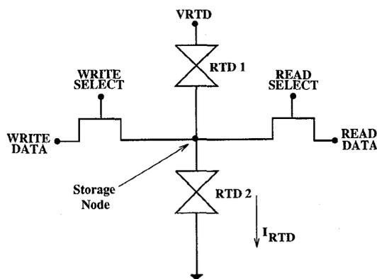
Figure 1: Schematic of an RTD/EFET SRAM cell.
