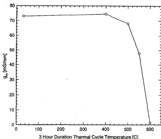
Figure 5: The maximum transconductance,  $g_m$  ( $V_{DS} = 0.15$  V), of fully processed  $50 \mu\text{m} \times 1.2 \mu\text{m}$  gate E-mode MESFETs after 3 hour anneals at temperatures between  $400^\circ\text{C}$  and  $600^\circ\text{C}$ .
