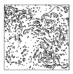
Figure 4: Wide range of interfacial scales seen in the case of phase inversion in a closed box from Figure 8 of Labourasse et al. (2007).
