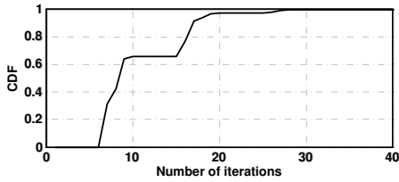
Figure 13: CDF of Algorithm convergence on hardware. About 30% of the runs have to recover from noisy minimas, but do so quickly.
