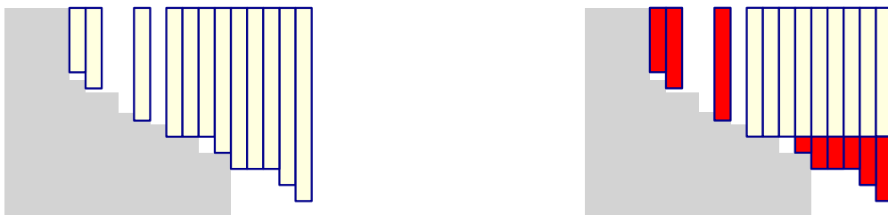
(a) A greedy packing of instance \mathcal{I}' . Large items are packed “on top” of the small items (in grey). (b) Packing of instance \mathcal{I}_\ell^k obtained from \mathcal{I}' by removing parts of huge items \mathcal{I}_\ell^k (in red).
