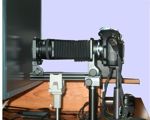
Figure 1. Nikon D100 digital camera with a customized lens and light baffle to measure the spatial distribution of light intensity produced by red, green, blue and white pixels. The lens is a 20 mm focal length objective placed in the reversed direction. In this position, the lens magnifies the pixels by a factor of 10 on the camera sensor.
