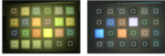
Figure 2. Raw camera images captured when the MCC is illuminated with the broadband “white” LEDs (shown on the left), and short wavelength “blue” LEDs (shown on the right). The rectangles superimposed on the images indicate the image area over which the mean R, G and B pixel responses were calculated. Many of the patches include fluorescent pigments that are visible when illuminated by the “blue” light. The fluorescence will also be present when illuminated by the “white” LED light, but the number of fluorescent photons is very low compared to the number of reflected photons.
