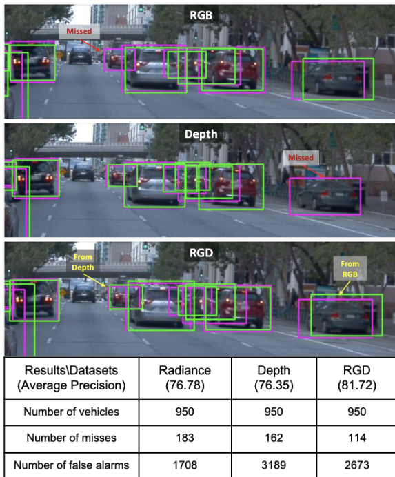
FIGURE 11. Vehicle detection examples from the Waymo dataset on a ResNet trained with radiance, depth or both. match the simulation analyses. Vehicles that were missed in RGB but found in depth, are also found in RGD. Similarly, vehicles that were found in RGB but missed in depth are found in RGD. Box outline colors as in Figure 8. The table shows the statistics of the detection results from radiance, depth and RGD networks.
