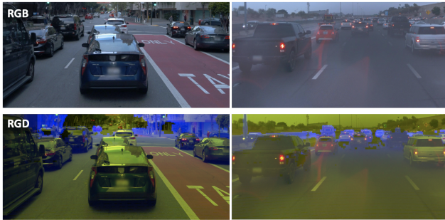
FIGURE 9. The two images at the top are radiance images from the Waymo dataset. The data set includes corresponding depth data. We combined the radiance and depth information into the two RGD images rendered at the bottom.
