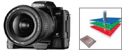
Figure 2. The Sigma SD9 is the first digital camera to use a full-color multi-layer sensor technology: The Foveon X3 sensor.
