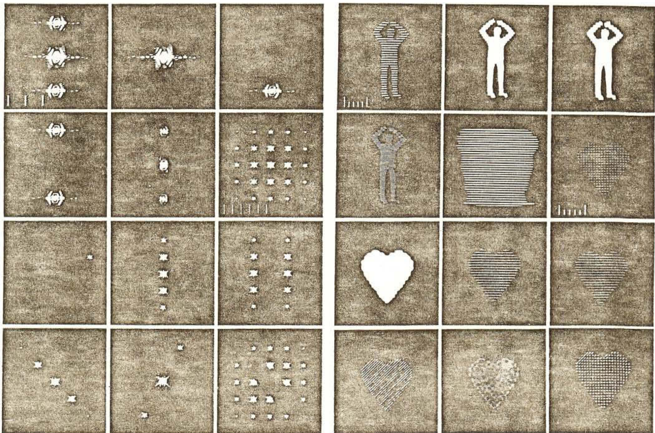
FIG. A6. Optical Fourier transforms. Each panel in the left block (three left-hand columns) shows the optical transform (i.e., amplitude spectrum) of the corresponding image in the right block (three right-hand columns). [From Harburn et al. (61). Reprinted from G. Harburn, C. A. Taylor, and T. R. Welberry: Atlas of Optical Transforms . Copyright © 1975 by G. Bell and Sons, Ltd. Used by permission of the publisher, Cornell University Press.]
