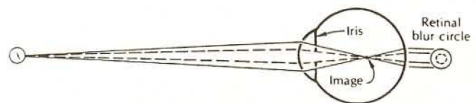
FIG. 1. Blur circles in a schematic misfocused eye for two different pupil sizes. [From Cornsweet (36).]
