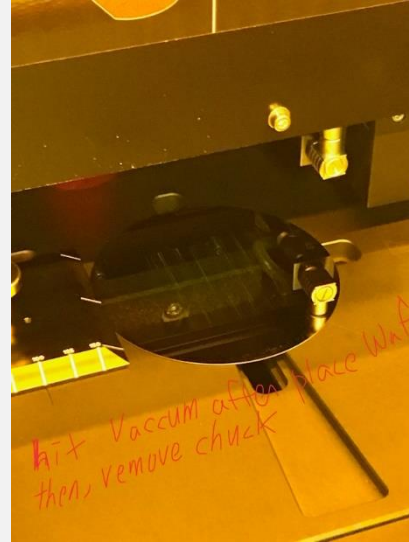
3- load resist-coated wafer, flat bottom attached to the chuck , do not worried about precision of the wafer location (MLA-150 automatically detect the center of wafer)
